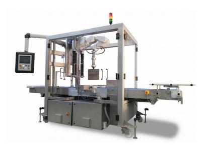
The robotic multifunction cell (IRM) is composed by a conveyor belt, an anthropomorphic robot completed with a portable control panel and has protections.
